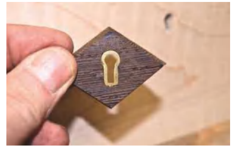
▲ Pic.15 The brass escutcheon is slightly tapered from the front narrowing to the back. After much filing, I finally got a tight fit
